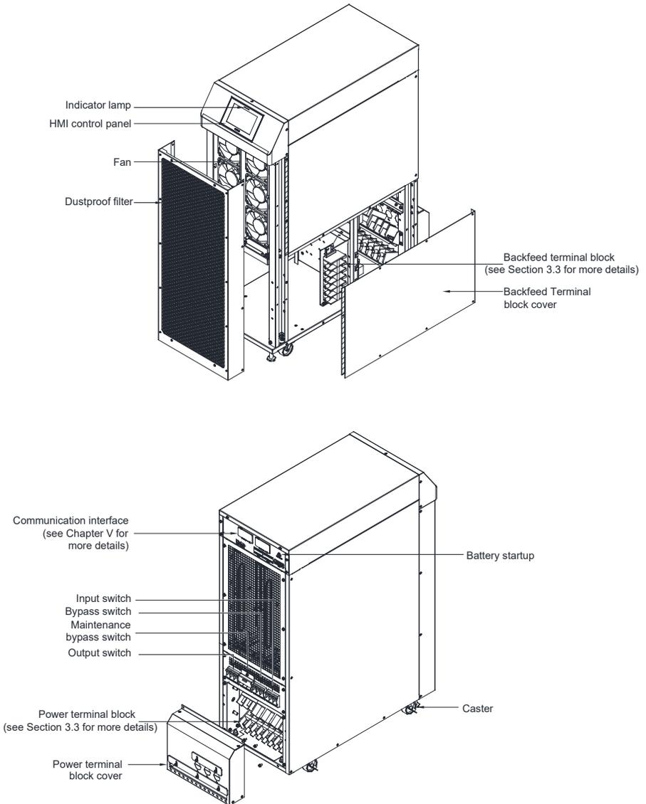
Figure 2-5: 60-80K structure diagram
