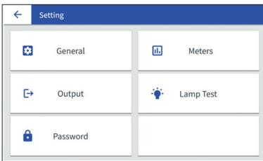
On the Setting interface, you can not only set the language, time, brightness, output voltage and frequency, but also modify the password. The menu structure of Setting is shown in the following table:
