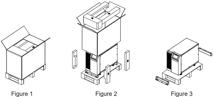
Figure 2-1:20-40K Unboxing diagram
