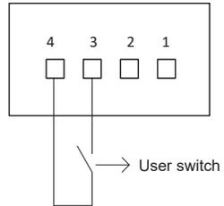
When 3-4 are closed, the UPS will perform emergency power off. 1-2 are idle.
