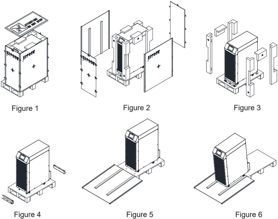
Figure 2-2: 60-80KS Unboxing diagram
