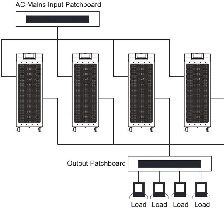
Figure 3-1: Parallel Installation
