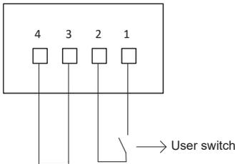
3-4 are connected with a short cable, and keep them connected. When 1-2 are open, the UPS will perform emergency power off
