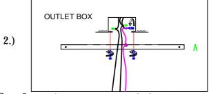
Step.2: Wire fixture to wires in outlet box. Green wire is for Ground.
