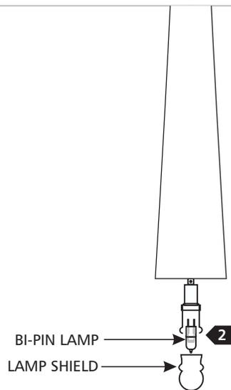
2 Remove the lamp shield and the old lamp.
