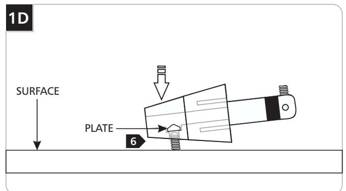
**6** Tap the conical connector on a hard surface with the set screw facing down, so the plate inside drops into place.
