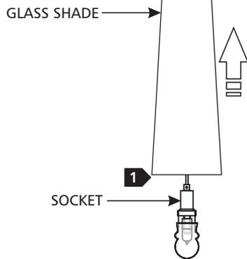
**CAUTION:** To reduce the risk of a burn or electric shock when replacing the lamp, disconnect the power to the fixture.
