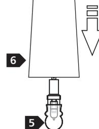
5 Push the lamp shield onto the spring clip.
