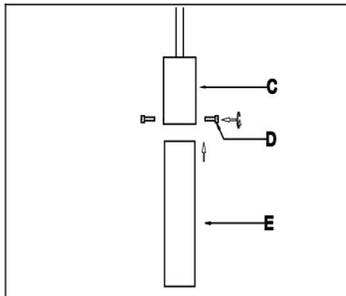
**Step 5. Insert glass (E) into cup (C) and secure using screws (D) provided**
