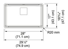
Pescara sinks are equipped with a level of functionality and performance that maximizes usability for the home chef or kitchen connoisseur. Crafted from 18-gauge stainless steel with smooth corners, this sink is low maintenance and easier to clean.
