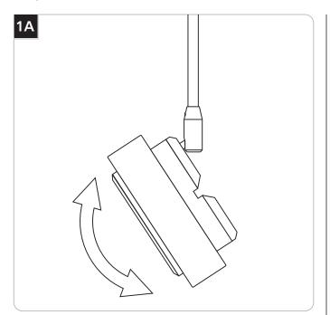
1 Tilt the fixture head to the desired position.
