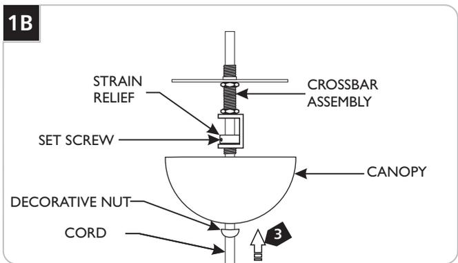
**2** Loosen (**Do Not Remove**) set screw in the strain relief.
