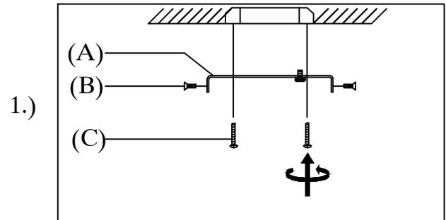
Step1 :Remove mounting bracket from fixture and install to electrical box.
