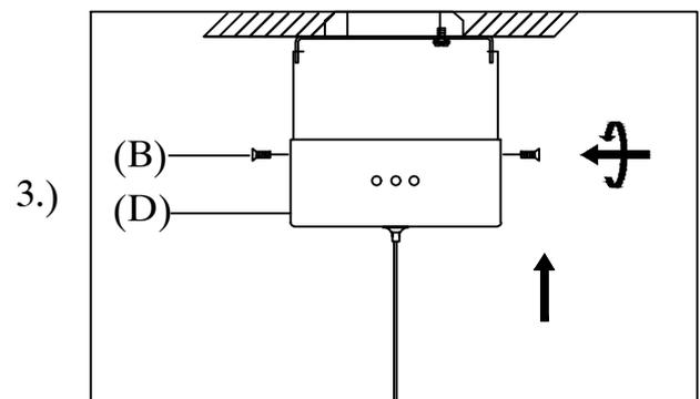
Step3 :Install fixture to bracket and Screws at the ends of the canopy to secure.
