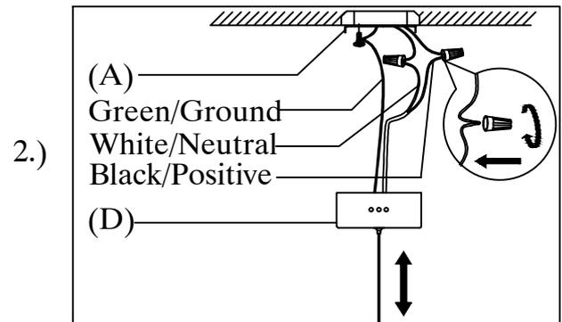
Step2 :Adjust wire length to desired mounting height, and tighten strain relief screws to secure. Wire fixture to wires in outlet box. Green wire is for Ground.
