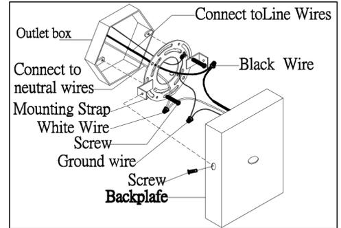
**Step.1:** Remove mounting bracket from fixture and install to electrical box. Then wire fixture to wires in outlet box. Copper wire is for Ground. Attach back plate to ceiling and tighten screws on the sides until fixture meets wall.
