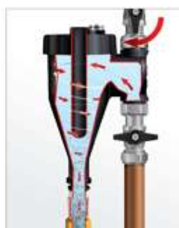
3. Open outlet and drain valves
