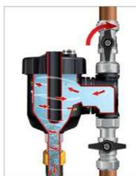
3. Open outlet and drain valves
