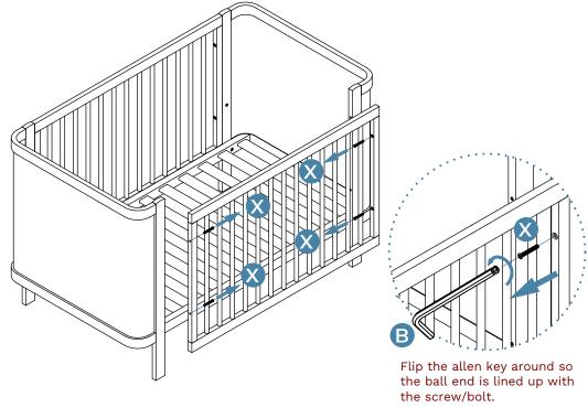
Remove the (X) Bolts already installed in the cot with Allen Key (B). Please hold onto the (X) Bolts as you will need these to install the conversion.
