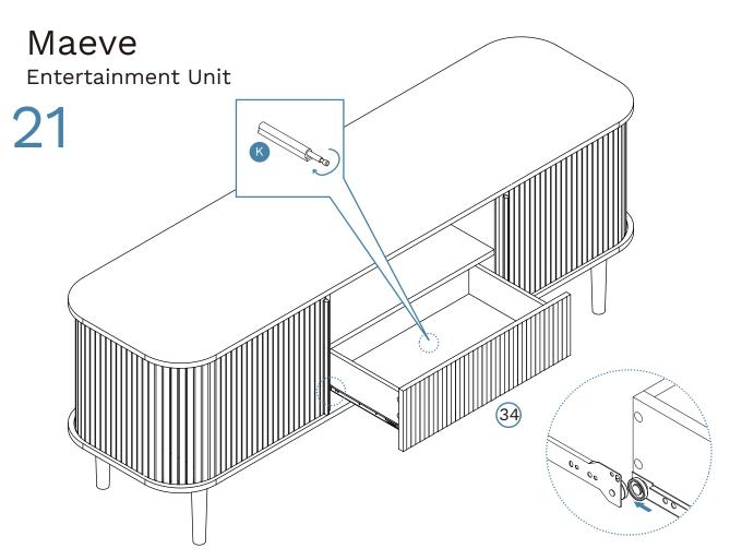
Insert the assembled drawers into the corresponding compartments as shown. Ensure the drawers slide easily along the rails. If the door is not catching or sitting flush, twist the end of the cover (K) until it catches on the seal (L).
