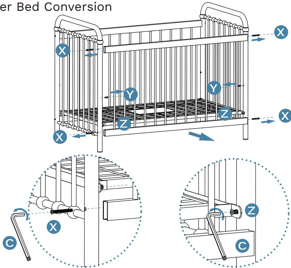
Remove the (X,Y) screws already installed in the cot with Allen Key (C). Loosen the screw (Z), don't all shake out. Please hold onto the (X) and (Y) screws as you will need these to install the conversion.
