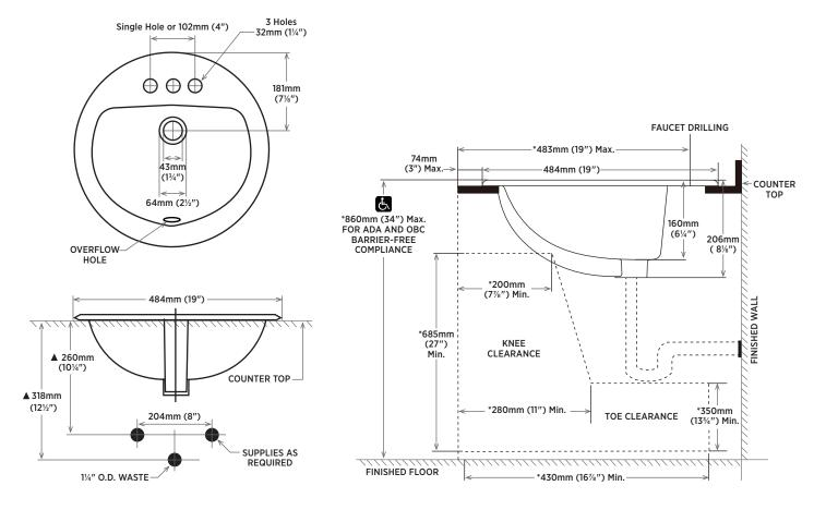
**NOTE:** \* Starred measurements comply with ADA and OBC barrier free accessibility requirements. Dimensions shown for location of supplied and waste are suggested.
