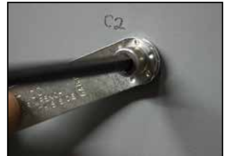
13d & e - With pressure on wrench tighten screw
