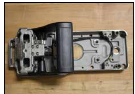
12 - Base Plate with both covers removed
