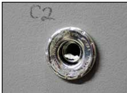
13f - Jack Nut firmly seated, screw removed
