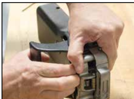
12b - Remove the larger portion of the cover off second.
