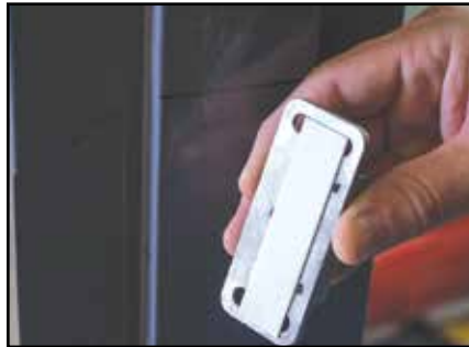
1c - Attach double stick tape to the back of the strike.
