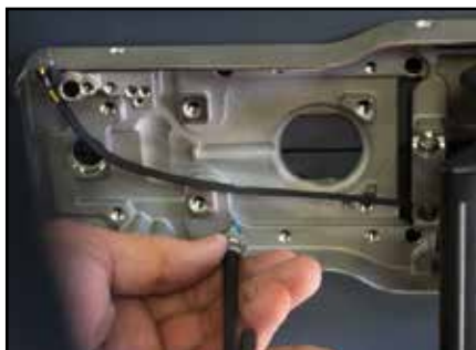
15c - Insert the (4) 1/4"-20x1-1/8" screws and split washers into the (4) B holes.
