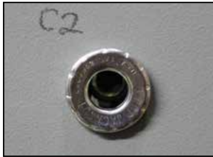
13a - Insert Jack Nut into C2 hole
