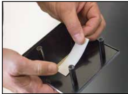
Tip - Use a piece of double-sided tape to hold the Exterior Trim Plate into place
