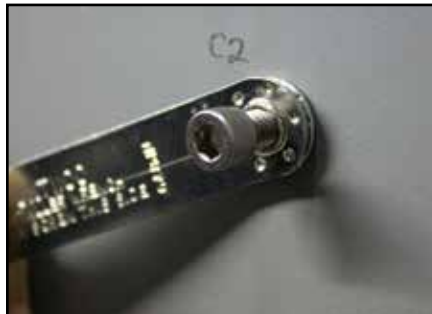
13c - Thread screw into Jack Nut until flush
