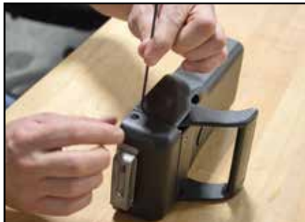
12a - Remove ALL (8) flat head back cover screws.
