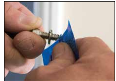
15b - Apply Thread Locker
