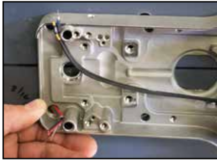
14a - Make sure you pull all wire through the optional (F) hole on the Base Plate if drilled
