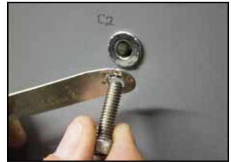
13b - Insert screw into Jack Nut Wrench
