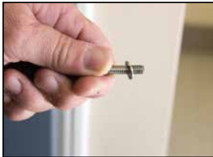
15a - Put split washer onto (4) 1/4"-20x1-1/8" socket head machine screws.
