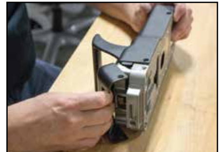
12b - Slide the smaller “nose cone” cover off first.
