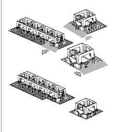
STEP 5. CONNECT THE FRAMES BY PRESSING THE SNAP FEATURES INTO EACH OTHER
