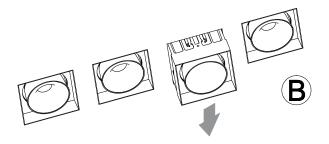
Pull module down out of the mounting kit for relamping or power supply changing
