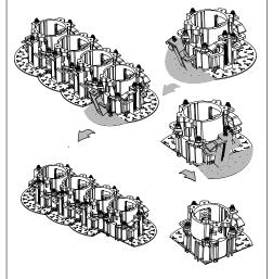
STEP 5. CONNECT THE FRAMES BY PRESSING THE SNAP FEATURES INTO EACH OTHER
