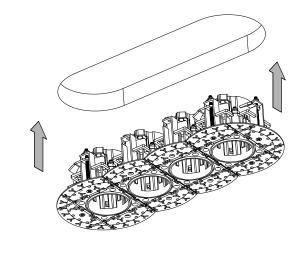
CEILING THICKNESS BETWEEN 2mm - 28mm
