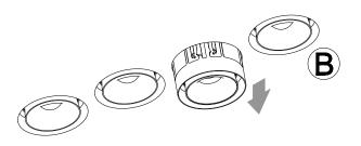
Pull module down out of the mounting kit for relamping or power supply changing
