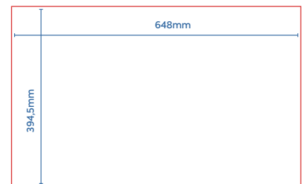
Required cut-out for the elevator panel
